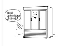
■ Set the front of the refrigerator a little bit higher than back-side by using adjustable feet to drain the water away with easily.
